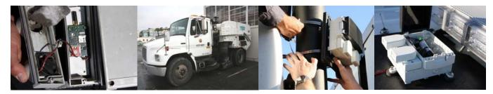
Figure 2. Variants of the sensing platform, enclosure-mounted on city street sweeping vehicles.
